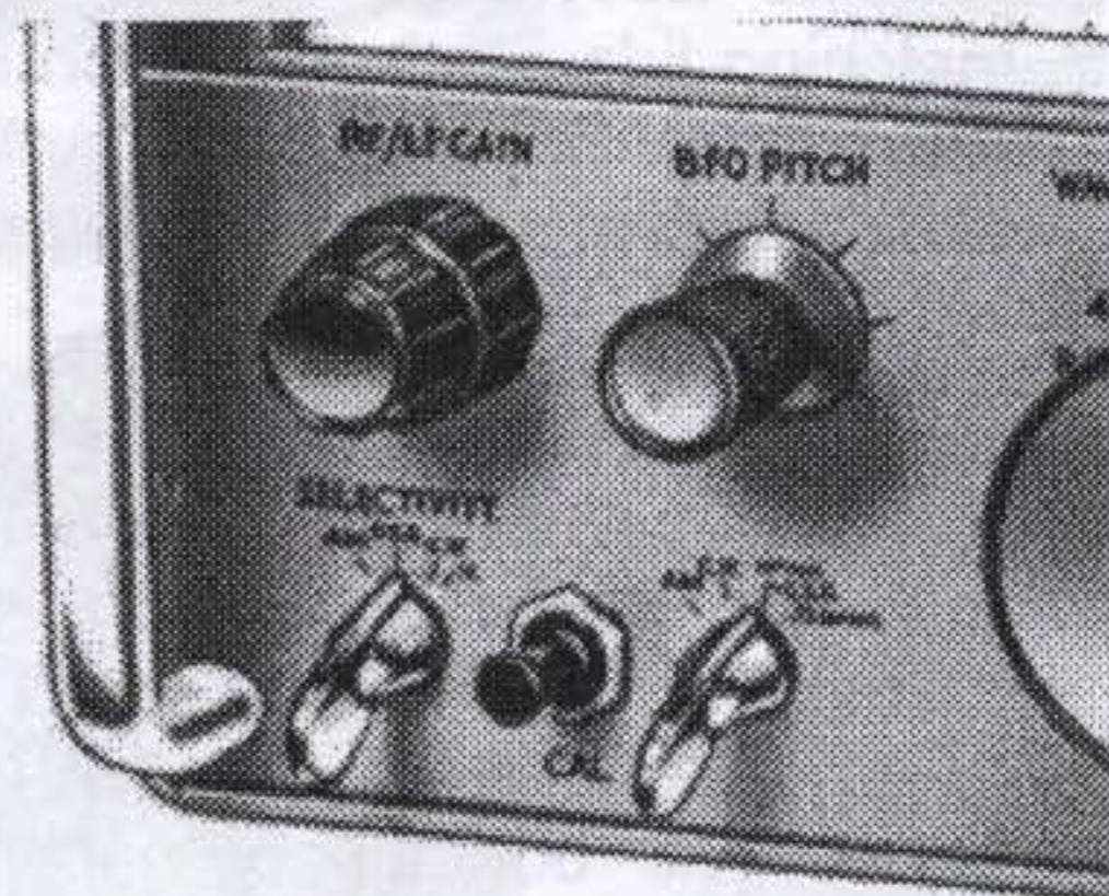
All the model 830-series had an odd pair of concentric knobs for the RF/IF gain controls.
